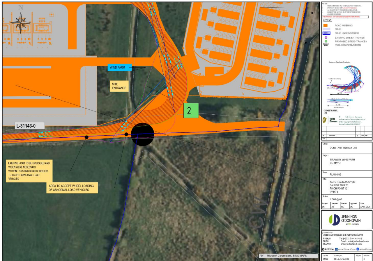
Figure 25: Auto Track Analysis Ballina to the Wind Farm Site Pinch Point 12
